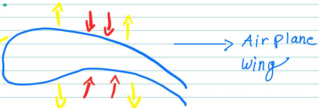
As we can see the Air plane wing is shaped in a special way that will increase the **Velocity** of Air on the upper part and decrease the **Velocity** on the lower part.
